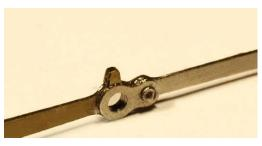
8. The rear length of each rod has a knuckle joint to manufacture. The front and rear rods are joined with a small rivet pushed through from the front and then cropped back on the rear leaving about 0.5 mm proud. See photo.
