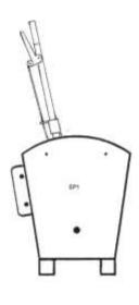
MICROSWITCH BRACKET MOUNTED ON REAR OF LEVER FRAME. PIVOT P1 ASSEMBLED AS SHOWN ON ABOVE DRAWING.
