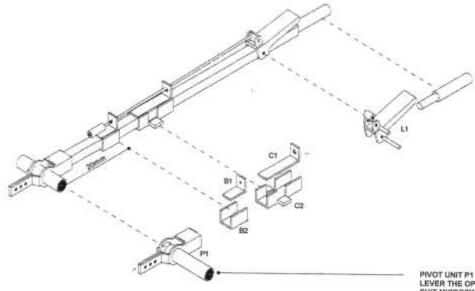
PIVOT UNIT P1 ATTACHED TO THE LEVER THE OPPOSITE WAY UP, TO SUIT MICROSWITCHES MOUNTED ON THE REAR OF LEVER FRAME. SEE INSTRUCTION 2.6
