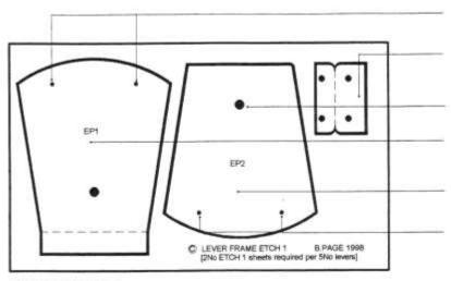
HOLES TO RECEIVE 0.7mm HARD BRASS WIRE TO ASSIST LOCATION OF FORMERS F1 AND F2
